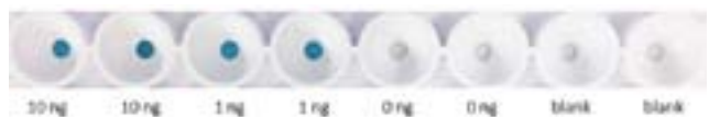
Figure 3. Different amounts of antigen give different results. Note that while the dot blot assay can easily distinguish between negative (0 ng) and positive (10 ng), it has more difficulty in distinguishing between 1 ng and 10 ng of antigens that were bound to the matrix.
