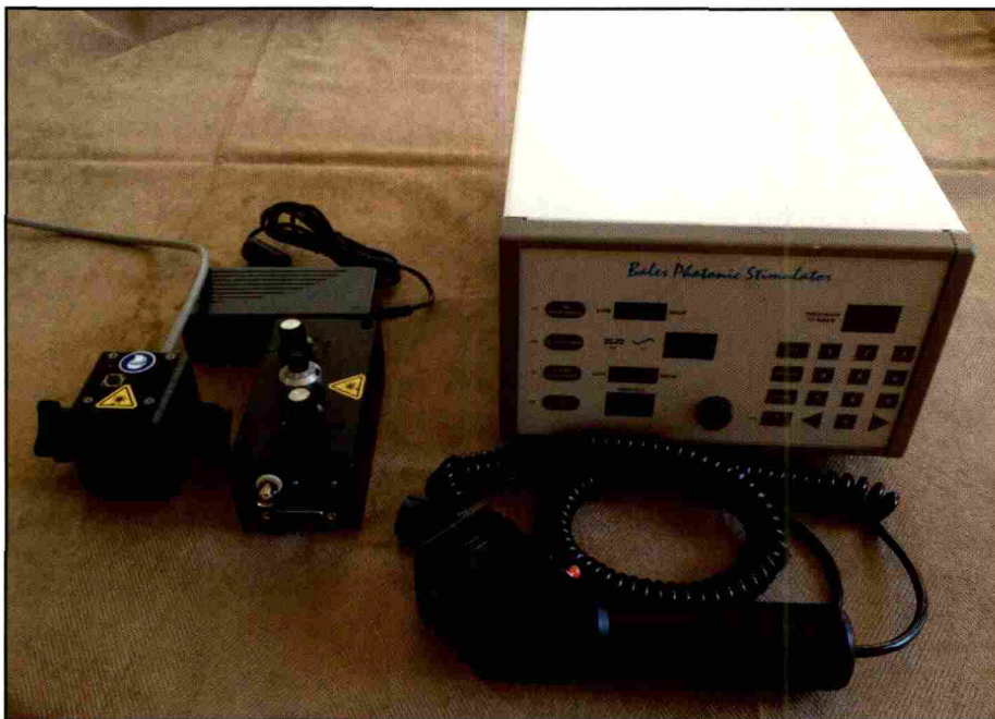
The light emitter, computer, and power supply of the new BioPhoton 100 on the left, compared with the original Photonic Stimulator on the right.
