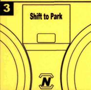
Car wash mode is set when [N] and "Shift to Park" is shown on the gauge. You will have 15 minutes before it will automatically shift to [P]. You may now exit the vehicle.
